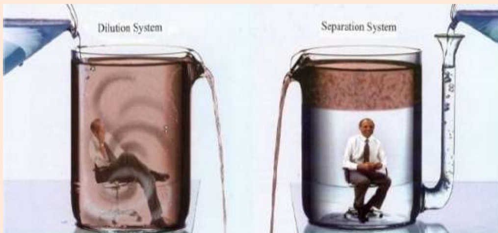
Figure 10: Office stale air dilution (conventional HVAC systems) vs separation (underfloor air displacement systems)
